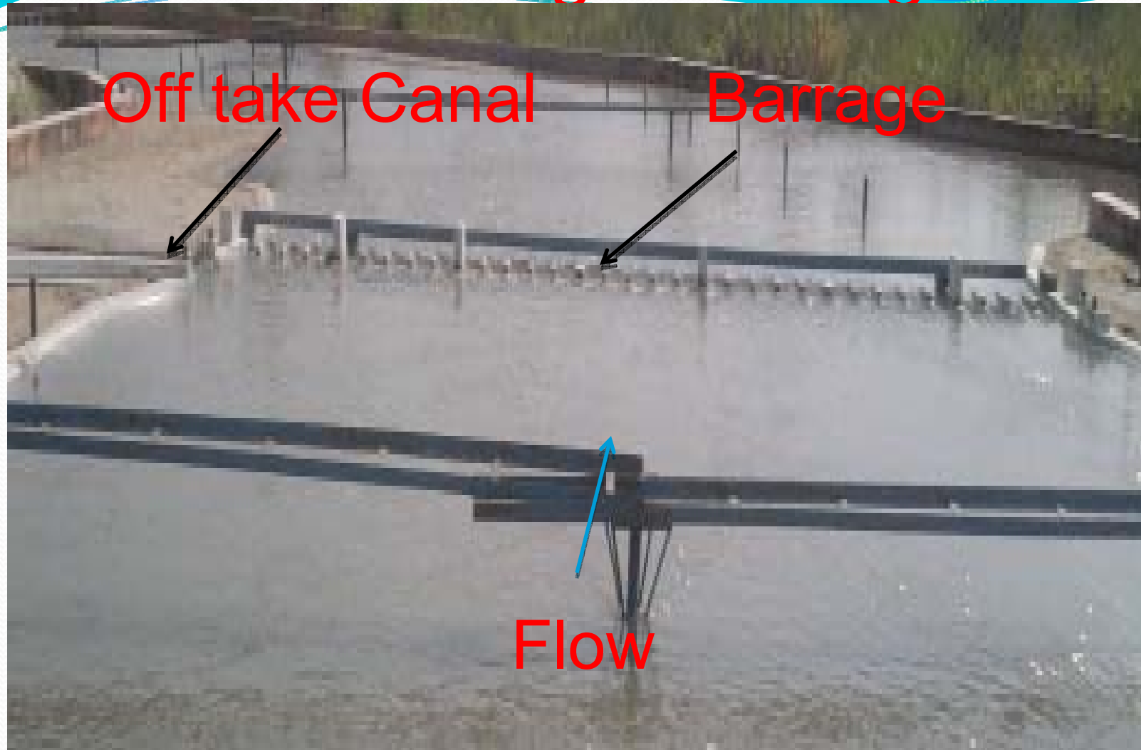
Model of Anandpur Barrage on river Baitarni (Odisha)
