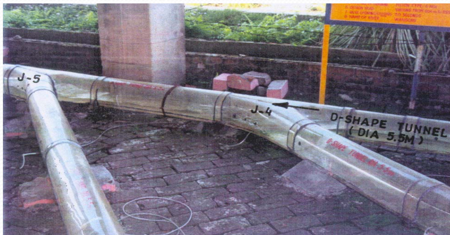
Model of Tail Race Manifold System
