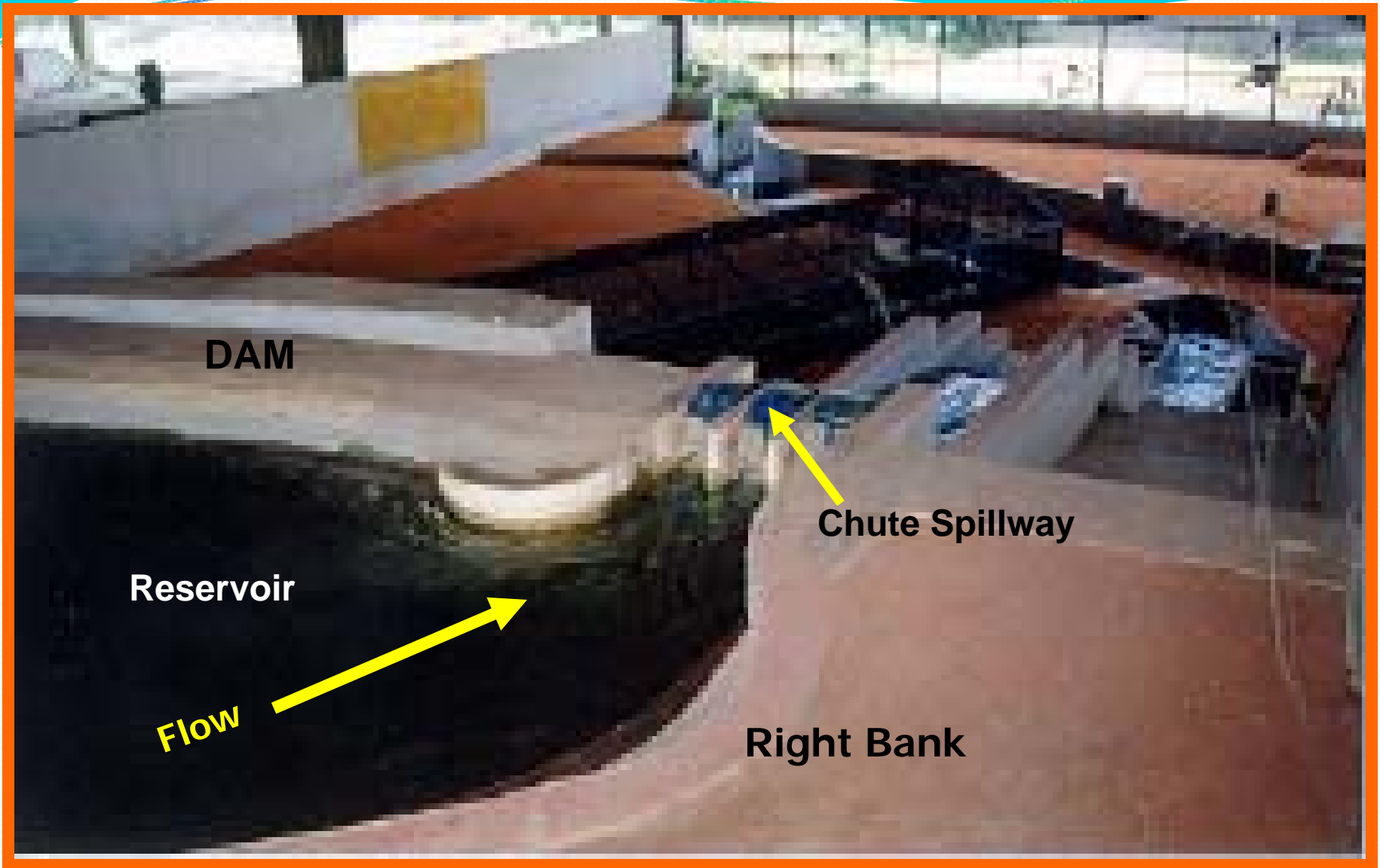
Top View of 260.5 m high Tehri Dam Model
